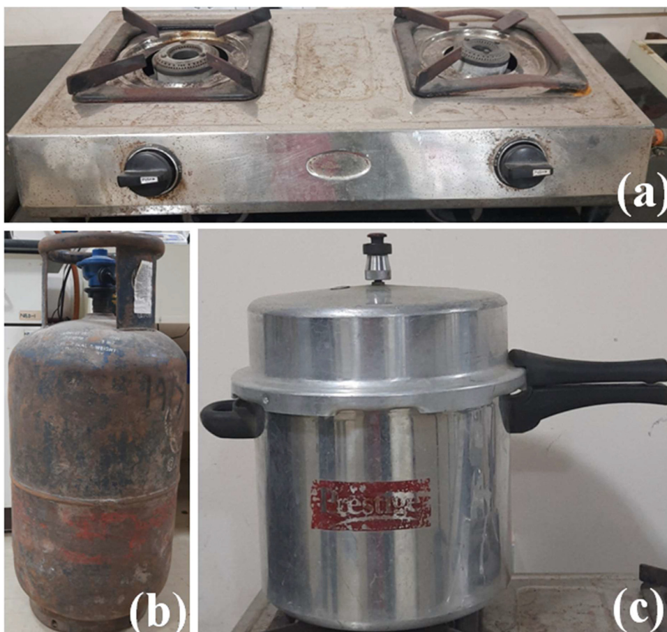
Fig. 2. Photographs of the apparatus and accessories used for the Ag NP synthesis, (a) LPG stove, (b) LPG cylinder and (c) domestic, LPG stovetop pressure cooker.
