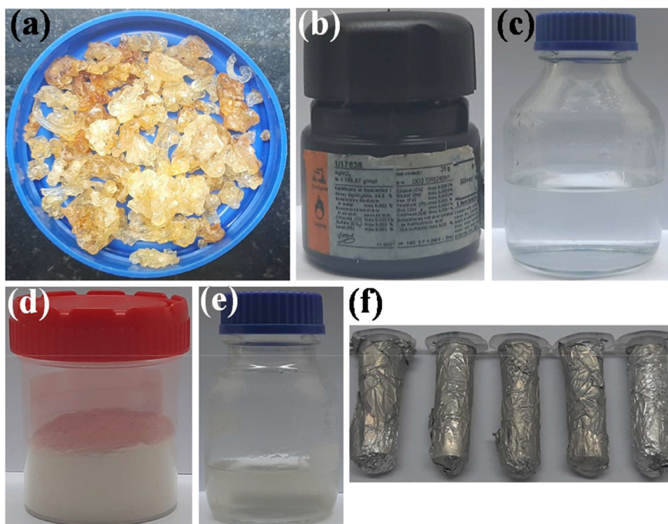
Fig. 1. Photographs of the materials used for the Ag NP synthesis by pressure cooker autoclaving, (a) gum kondagogu, (b) silver nitrate (c) ultrapure water, (d) powdered gum, (e) 0.5 % gum solution and (d) 100 mM stock solutions of silver nitrate in small vials.
