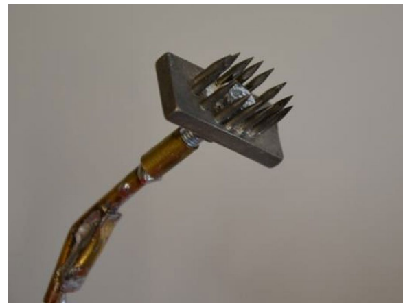
Fig. 1 Pin-shaped electrodes (size: 1 \times 2 cm, pin length: 1 cm)
