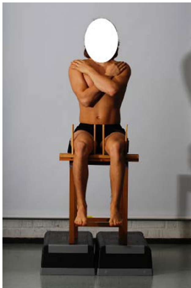
Figure 5 Participant sitting with a neutral posture, with both hips and knees at a 90° angle and the thighs held in position by four wooden bolsters to prevent hip abduction/adduction translation.
