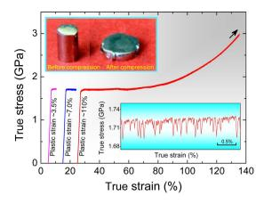
Figure 2. True stress-strain curves of Z2 uniaxially compressed to different plastic strains at room temperature (curves are shifted to the right for clarity). The top-left inset shows a Z2 specimen before and after compression to 110% plastic strain. The bottom-right inset shows a magnified view of the serrated flow in the plastic regime.
