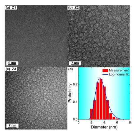
Figure 1. HRTEM micrographs of as-cast specimens. (a)  $Z1 - (Fe_{0.6}Cu_{0.4})_{33}Al_8Zr_{59}$ , (b)  $Z2 - (Fe_{0.45}Cu_{0.55})_{33}$   $Al_8Zr_{59}$ , and (c)  $Z3 - (Fe_{0.3}Cu_{0.7})_{33}Al_8Zr_{59}$ . Panel (d) shows the size distribution for the glassy nanospheres in ascast Z2.
