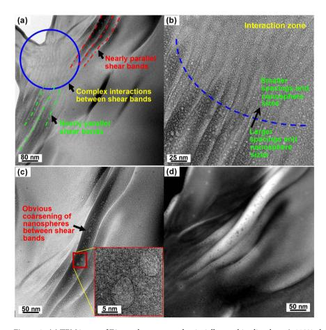
Figure 4. (a) TEM image of Z2 sample compressed uniaxially to a thin-disc shape (~110% plastic strain, Fig. 2), showing numerous shear bands (lines) and an interaction zone (circle). (b,c) HRTEM micrographs of the shear bands near the green and red lines in (a). The inset in (c) is a higher-magnification image of the region marked by the red rectangle. (d) STEM image corresponding to the TEM image in (c), further verifying chemical heterogeneity.
