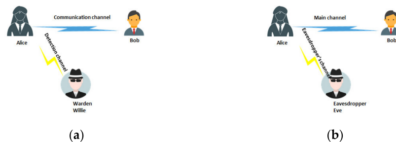
Figure 6. Difference between low probability of detection (LPD) (a) and physical layer security (PLS) (b).
