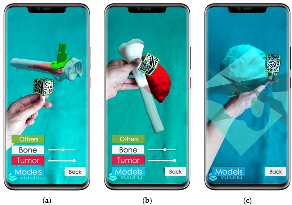
Figure 4. ARHealth smartphone application. (a) Demo mode using patient AR3DP0005 3D models, tumor is represented in red inside the bone, which is displayed in white with transparency texture; (b) Virtual visualization (tumor in red, bone in white with transparency texture) overlaid on top of the 3D-printed bone fragment (solid white) of patient AR3DP0007 using Clinic mode; (c) Surgical mode visualization of patient AR3DP0004 (tumor is represented in blue and cutting planes in semi-transparent green). A green frame surrounding the AR marker indicates that the reference is being tracked by the system.
