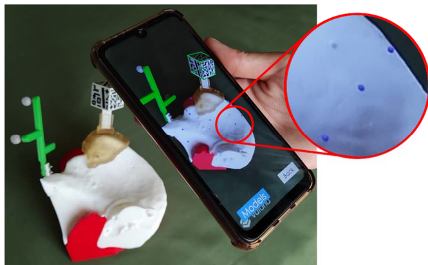
Figure 6. Phantom of patient AR3DP0002 (buttock tumor) and smartphone with the ARHealth validation app. The Augmented Reality Tracking Error validation spheres are augmented on the phantom surface in deep blue.
