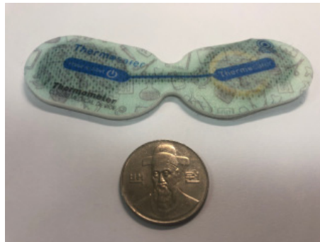
Figure 1. We use a wearable sensor which includes a thermometer and a 3-axis accelerometer along with Bluetooth transmission capability.
