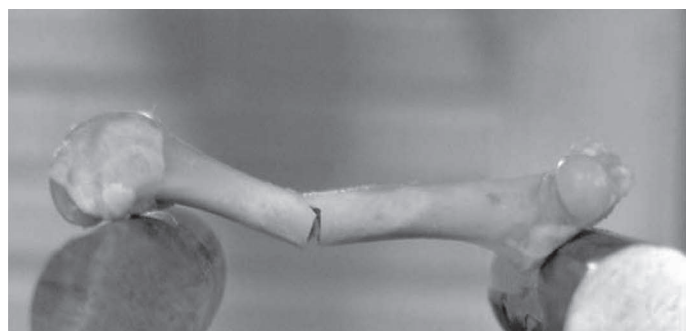
Figure 3 – Demonstration of specimen positioning in the test apparatus for producing fractures (left) and fracture pattern obtained (right)
