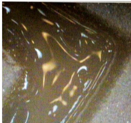
Figure 6. Optical microscope image of melt glass frit obtained with laser scanning.
