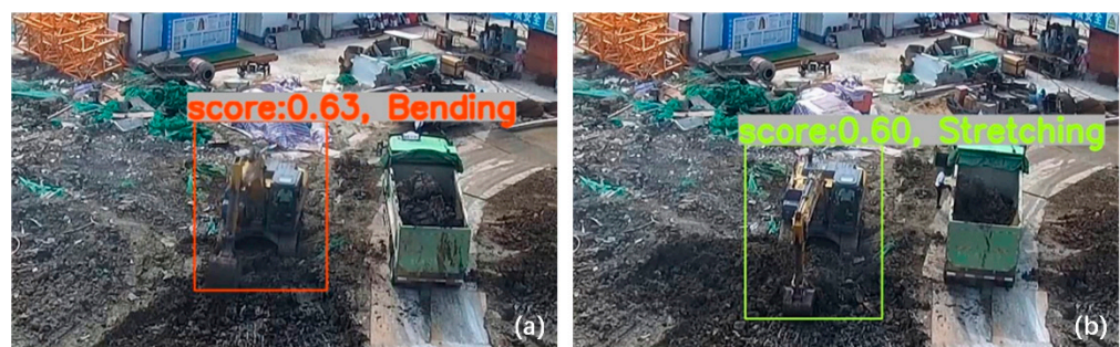
Figure 7. Wrong atomic action recognition. (a) “Stretching” is recognized incorrectly as “Bending”; (b) “Bending” is recognized incorrectly as “Stretching”.
