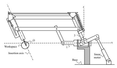
**Figure 3.** Candidate architecture in tilted position, where the numbers represent the names of the rods, and the letters the names of the rotation axes.
