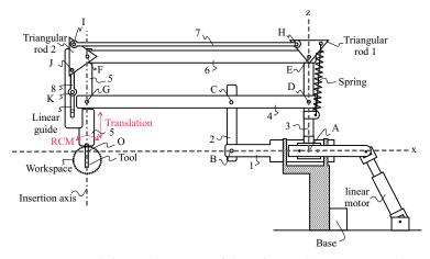
**Figure 2.** Candidate architecture of the robot with its security, where the numbers represent the names of the rods, and the letters the names of the rotation axes.
