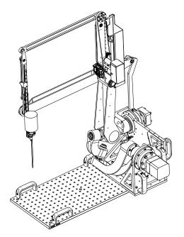
Figure 4. Prototype of the robot with an RCM.
