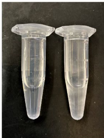
Supplementary Figure 15. The wet strength test of EV sheets (Lt) or normal pulp paper (Rt). The normal paper fibers unravel, and the solution becomes cloudy.
