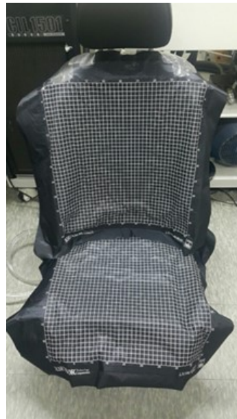
Figure 14. Pressure mat setting with SSA seats.
