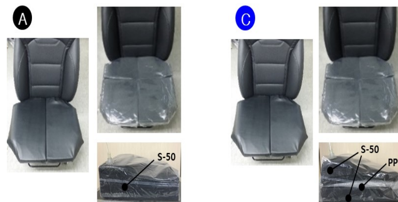
Figure 17. Configuration of pan layer of SSA seats (only for Model A and C).
