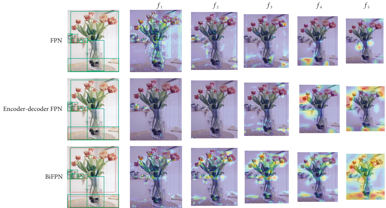
FIGURE 1: Heatmap visualization examples of current fusion methods. f_i, i = 1 \dots 5 , means the output feature of i -th level in pyramid network. Green boxes: ground truth; red boxes: detection result.
