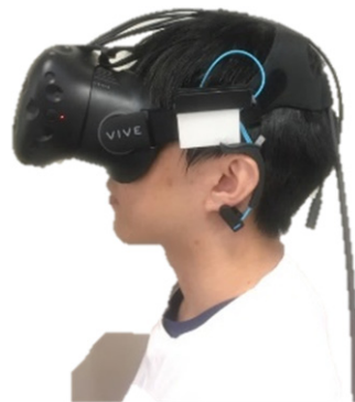
Figure 2. The VR HMD with the attached EEG sensor.
