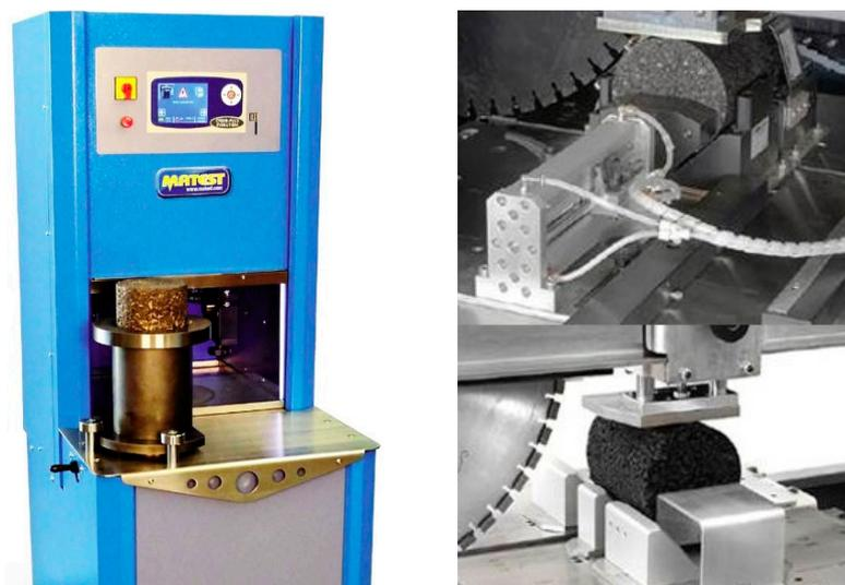
**Figure 3.** Gyratory compactor device and test specimens.
