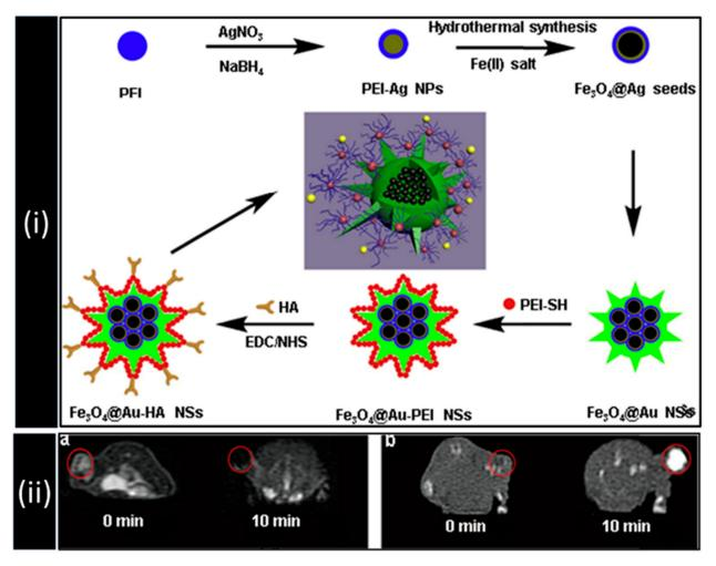
**Figure 7.** (i): Schematic illustration of the synthesis of Fe<sub>3</sub>O<sub>4</sub>@Au- hyaluronic acid (HA) nanostars (NSs). (ii): (a) T<sub>2</sub>-weighted MRI scan and (b) CT images of the tumors in a xenografted tumor model before injection and 10 min post intratumoral injection of nanocomposites. Red circles in Figure 7ii represent selected tumor sites. Reprinted with permission from ref. [69]. Copyright 2015 Elsevier.
