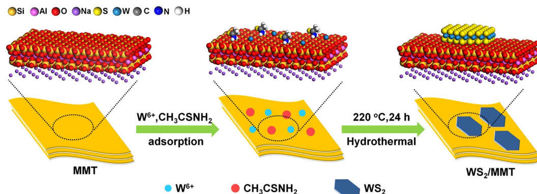
Figure 1. Schematic representation for the hydrothermal preparation of WS_2/MMT .
