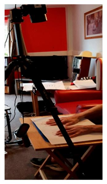
**Figure 1.** Long wave infrared imaging detector mounted on a tripod. The figure shows the participant during imaging with hands positioned upon a paper 'hand template' overlying an insulated tile. The portable table was used throughout the study to ensure consistency of the imaging set-up.
