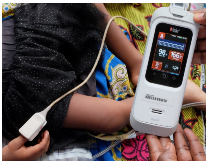
Figure 1. Automated respiratory rate counting with Masimo Rad G pulse oximeter. A one size fits all probe is attached to the thumb of a child admitted to Kisantu hospital with severe febrile illness. On the display, the plethysmogram is displayed on top, below the oxygen saturation of 98%, heart rate of 166/min and respiratory rate of 70/min are displayed. The heart rate and respiratory rate are too high and provoke a visual (red color) and sound alarm (silenced in the upper left corner).
