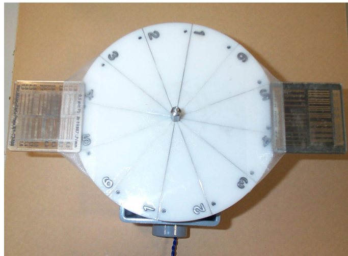
Fig. 4. The rotating spoke test pattern with two bar patterns (Nuclear Associates, NY) attached and the disk mounted on a rotating gear drive motor
