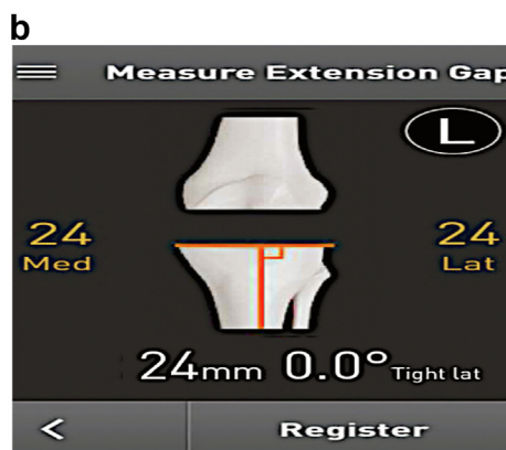
The OrthAlign gap tensioner was reinserted after performing additional medial release, demonstrating equal medial and lateral extension gaps.
