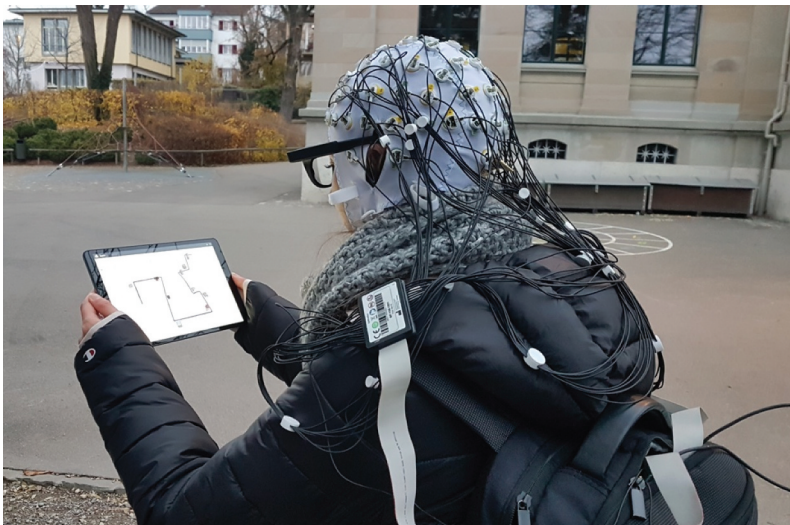
Figure 5. Real-time ambulatory assessment of a navigator's visual attention (mET) and cognitive load (mEEG) during mGID-assisted wayfinding task outdoors [image source: Armand Kapaj].
