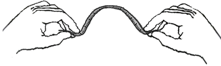
FIGURE 3: A flexible beam represented by a metal measure tape is held tightly on both of its ends. In order to pull the tape upwards an extra force is required to overcome the friction. Spontaneous straightening of the beam is not possible because its shear force is insufficient to overcome friction at the side points. Therefore, if no movement occurs at the side points, no force will be delivered by the beam at the midpoint.
