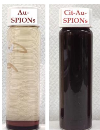
Figure A2. Dispersion stability of Au-SPIONs and Cit-Au-SPIONs after one week of storage at 4 °C.
