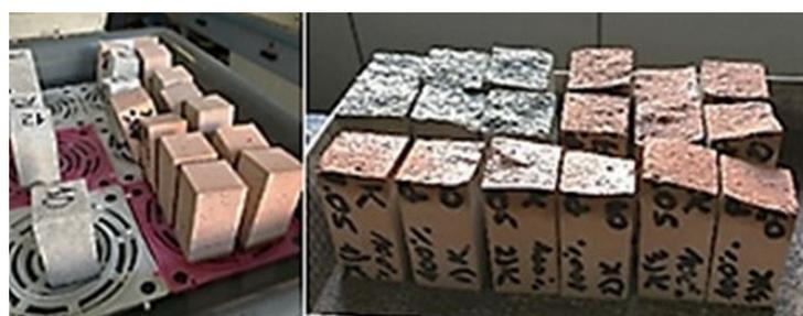
**Figure 6.** Determination of the water absorption due to capillary action.
