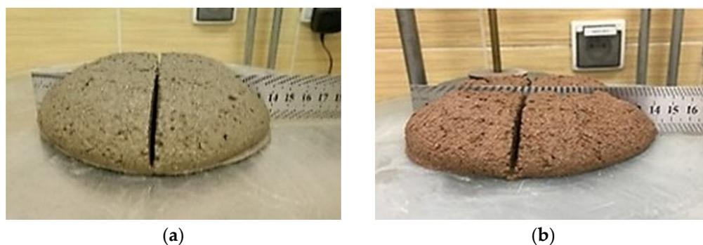
**Figure 3.** Measurements of consistency in a slump flow test. (a) reference mix; (b) mix with recycled ceramic waste M50.
