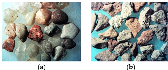
**Figure 4.** Aggregate grains of the 1.6/2.0 fraction (10×) (a) natural sand; (b) recycled ceramic waste.
