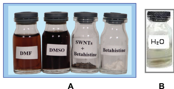
Figure 3 Solubility of grafted SWCNT–betahistine A ) in dimethylformamide (DMF) and dimethylsulfoxide (DMSO) and B ) in H_2O .
