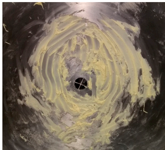
Figure 6. Deposited white chocolate fouling.
