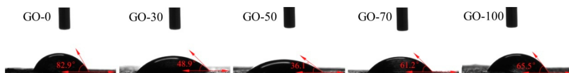
Figure 2. Contact angle of graphite oxide samples prepared at different reaction temperatures.
