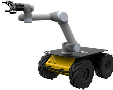
Fig. 2. Autonomous Ground Vehicle (AGV) with mounted serial manipulator [6].
