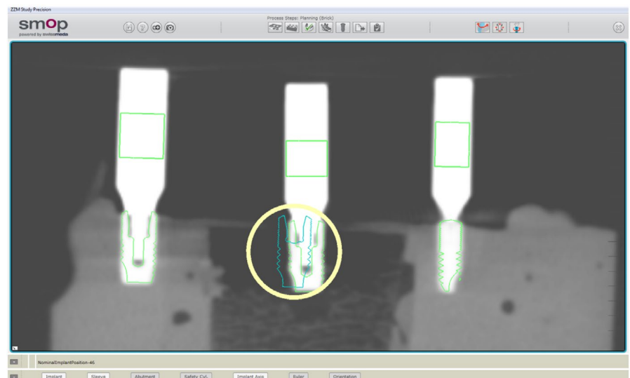
FIGURE 8 Direction of deviations: 1. Lateral horizontal deviation at the base of the implant, 2. Lateral horizontal deviation at the apex of the implant, 3. Vertical deviation, and 4. Angular deviation
