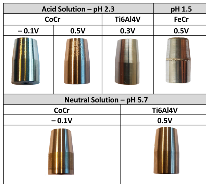
Figure 5. Pictures of the crevices of CoCr, Ti, and FeCr cones, after 1 month under crevice condition except for FeCr samples (2 days).
