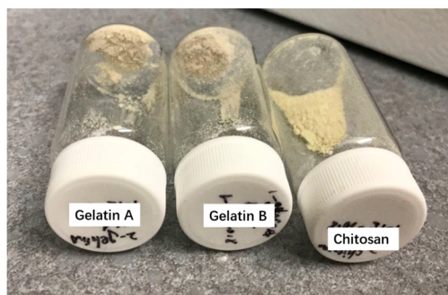
Figure 6. Comparison of gelatin- and chitosan-coated particles. Storage at 30 °C and 75% RH causes gelatin-coated particles to stick together and to the container, whereas chitosan-coated particles remain free-flowing.
