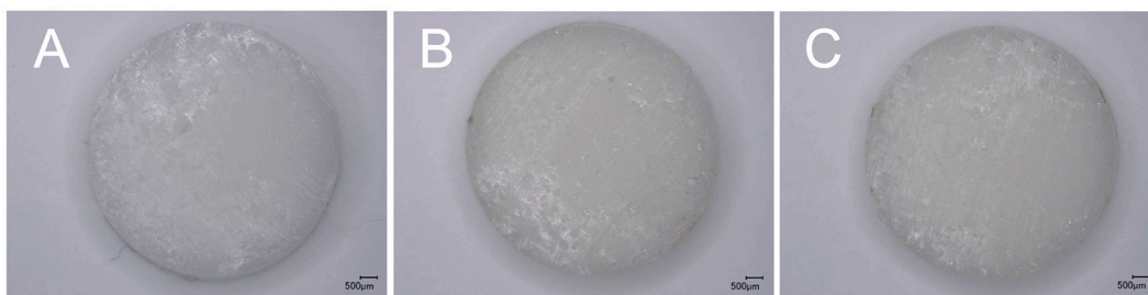
Fig. 6. Representative images of 200/320 mg DPV + LNG ring cross-sections (7.7. mm diameter): A – untreated control; B – exposed to SMF-only; C – exposed to SMF + 20 µM H 2 O 2 media for 30 days. Images were recorded using ×30 magnification.
