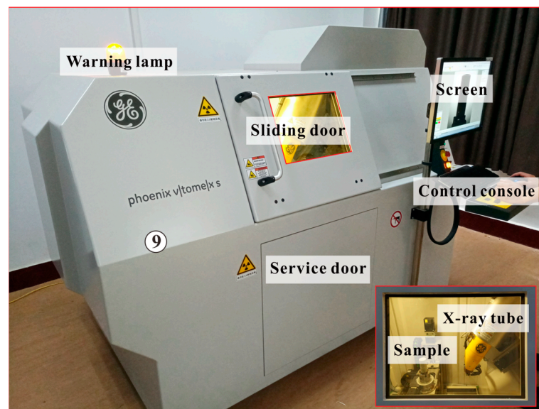
Figure 8. Apparatus for computed tomography (CT) test.
