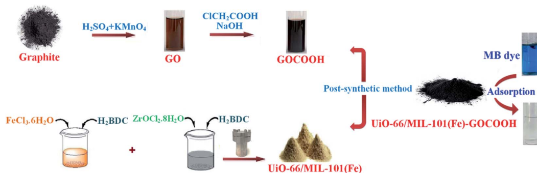
Fig. 1 Graphical diagram for the synthesis of UiO-66/MIL-101(Fe)-GOCOOH composite and photos for adsorption process.
