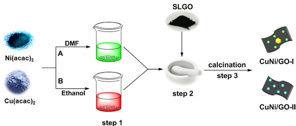
Scheme 1. Schematic illustration for the preparation of CuNi/GO-I and CuNi/GO-II.
