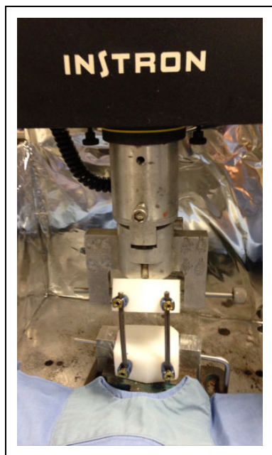
Figure 2. Nitinol construct (4 pedicle screws, 2 rods, and 2 polyethylene blocks) in testing apparatus with Instron.
