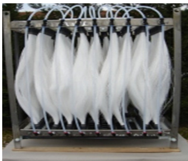
Figure 16. The permeation module ( 100 \text{ m}^2/\text{m}^3 ).
