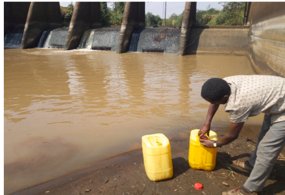
Fig. 2. Taking a sample from the intake of Jimma town water treatment plant.
