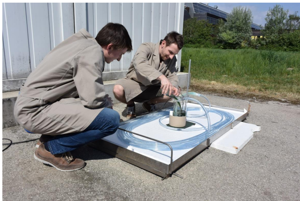
Figure A2. Inoculation of the 5-L tubular photobioreactor in Tulln with Synechocystis sp. IFA-3 for outdoors operation.
