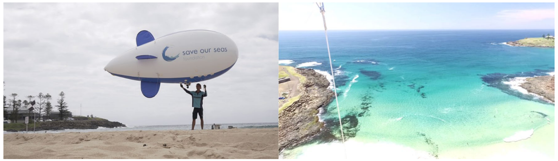
Figure 1. The blimp with camera module attached (left) and the view of Surf Beach from the blimp deployed at 70 m height.
