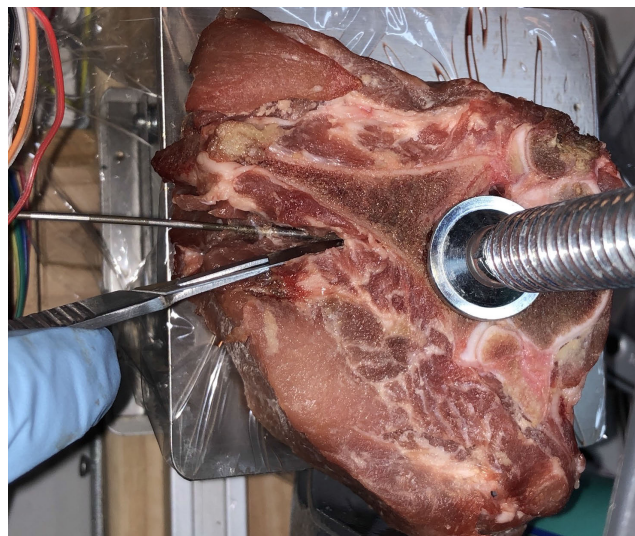
FIGURE 4. Dissection of test material with needle in place to verify bone strike.
