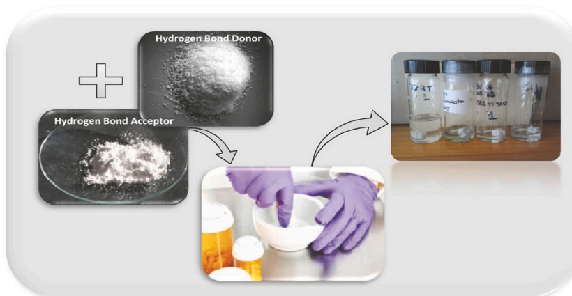
Fig. 4. Schematic representation of DES preparation using the grinding method. Reproduced with permission from Ref. [45].
