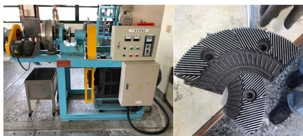
(A) Pilot-scale 12'' single-disc refiner (B) #005 knife plate
