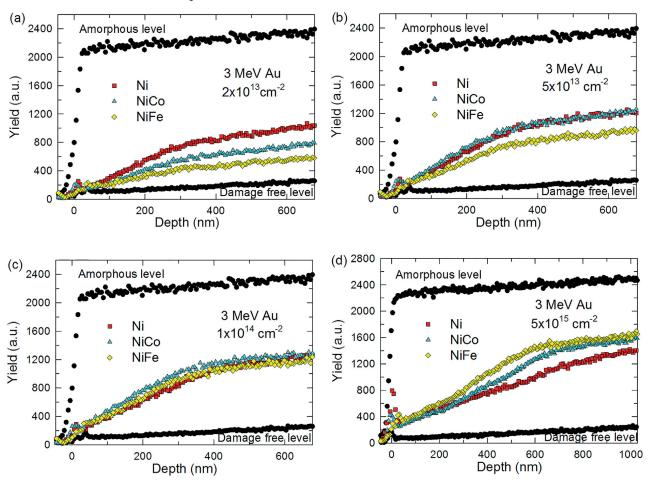
**Figure 3.** Rutherford backscattering channeling spectra of Ni , NiCo and NiFe, irradiated with 3 MeV Au ions to the fluences ranging from  $2 \times 10^{13}$  (a),  $5 \times 10^{13}$  (b),  $1 \times 10^{14}$  (c) to  $5 \times 10^{15}$  (d) ions cm<sup>-2</sup> Reproduced from Reference [80].
