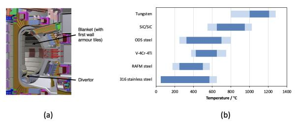
**Figure 1.** (a) Cross section of the ITER tokomak, showing location of first wall, blanket and divertor structures. (b) Operating temperature windows (based on radiation damage and thermal creep considerations) for selected fusion candidate materials. The light shaded bands on either side of the dark bands represent the uncertainties in the temperature limits. This figure is a modified version of that first presented in Reference [8].
