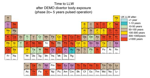
**Figure 2.** Periodic table of the calculated time period that each element would require to decay to UK low level waste limits ( $<4\,\mathrm{MBq\,kg^{-1}}$  alpha radiation and  $<12\,\mathrm{MBq\,kg^{-1}}$  combined gamma and beta radiation) following exposure inside a DEMO fusion reactor. The component considered is the divertor over a time period equivalent to 5 years of pulsed operation. Reproduced from Gilbert et al. [15].
