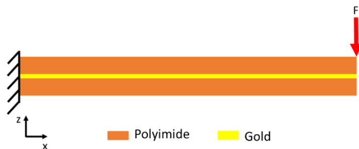
Figure 2. Schematic illustration of the mechanical model used to investigate the mechanical stress occurring as a result of bending.
