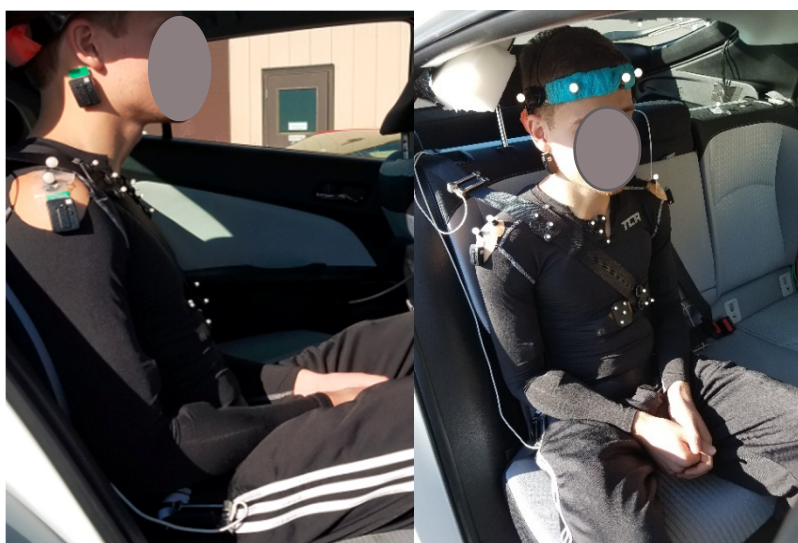
Figure 2. Subject instrumentation: photo-reflective markers placed on the head, the trunk, and the seat belt (left), and wireless EMG (electromyography) sensors visible on the neck and the right deltoid (right).
