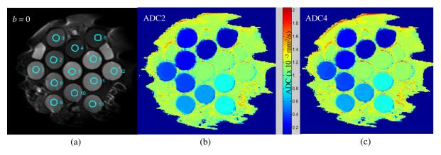
Fig. 1 (a) illustrates example screen-captures of a middle slice for T2-weighted image (with inscribed, numbered ROIs) for the PVP phantom (scanner 1 source, S1) and the corresponding (b) ADC2 and (c) ADC4 maps generated by "SW3" analysis. Two ROIs are defined for each %PVP > 0 concentration and three for ice-water (%PVP = 0). Common scale for the ADC2 and ADC4 maps is indicated by the color-bar between (b) and (c).
