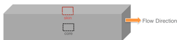
Figure 3. Illustration of injection-molded specimen with marked cutting positions for TEM investigations.
